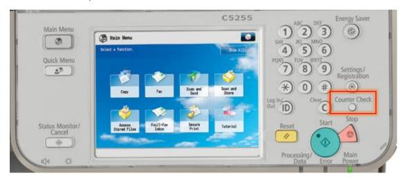
Once pressed the meter readings will be displayed on screen
